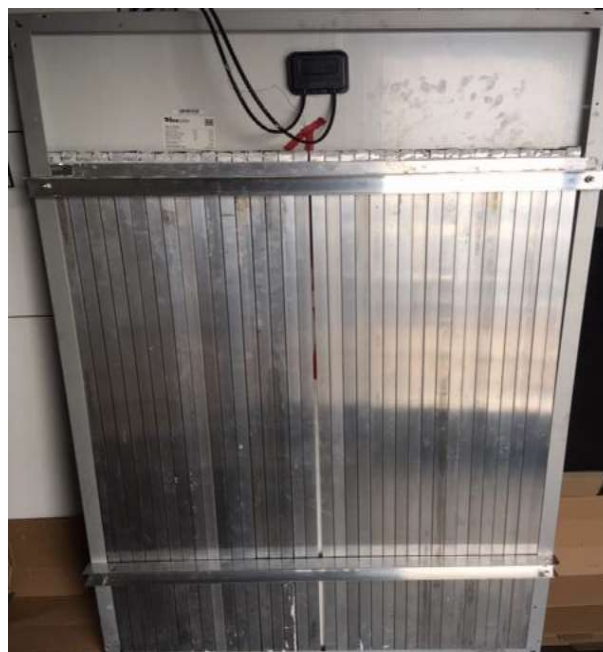
Figure 3.1.2.2. Aluminum PCM profiles arranged on the back of the panel (7)
