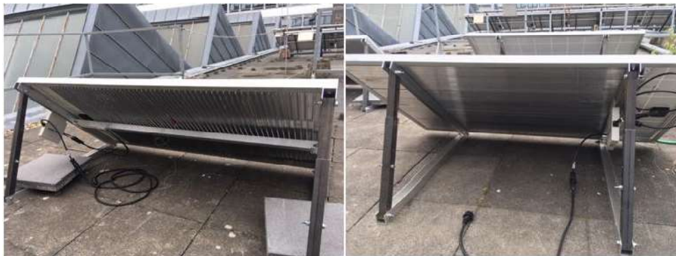
Figure 3.1.4. Cooling fins and PCM profiles coupled on the back of two of the installed PV panels (7)
