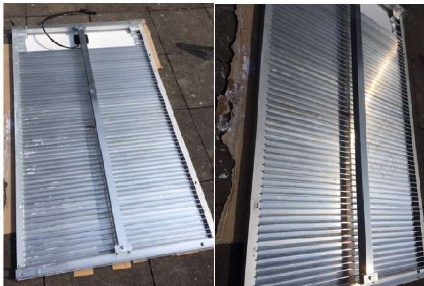
Figure 3.1.1.2. Aluminum fins arranged on the back of the panel (7)
