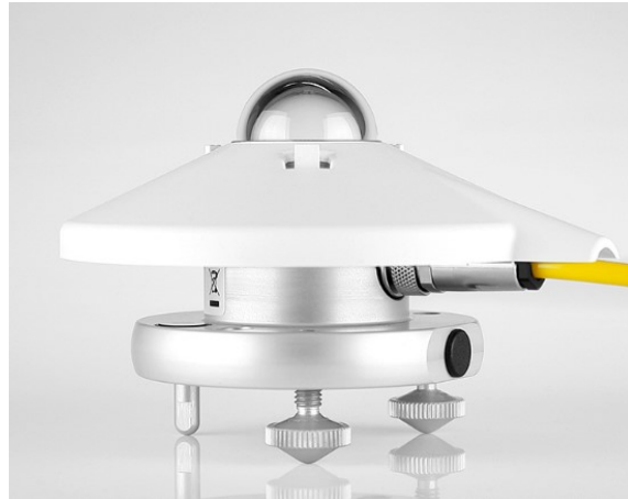
Figure 3.2.2.1. CMP3 Pyranometer of Kipp&Zonen (22)
