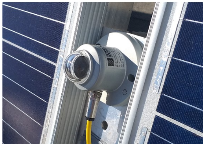
Figure 3.2.2.2. Pyranometer coupled on the top surface of the PV panels
