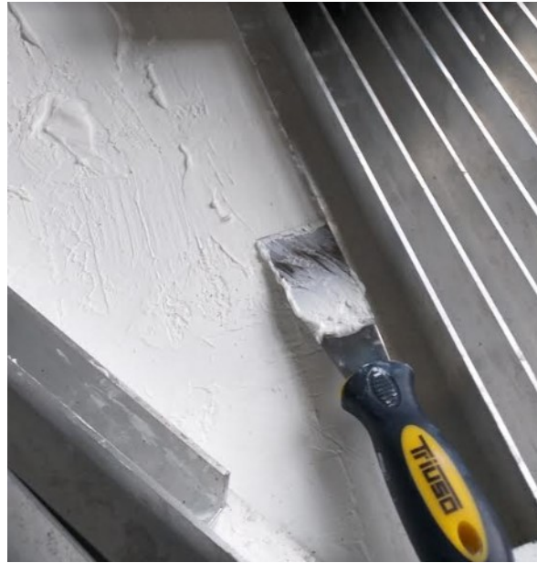
Figure 3.1.1.3. Application of thermal paste for a good thermal conductivity between the back of the panel and the aluminum fins
