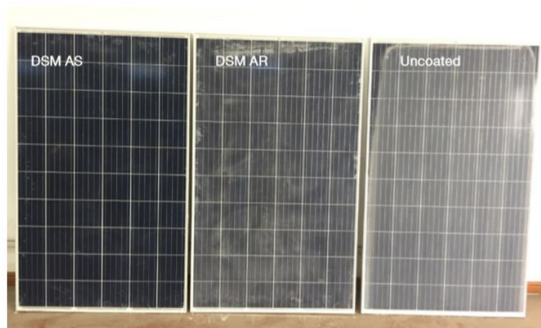
Example of soil-Performance difference between AR, AS and uncoated glass.
