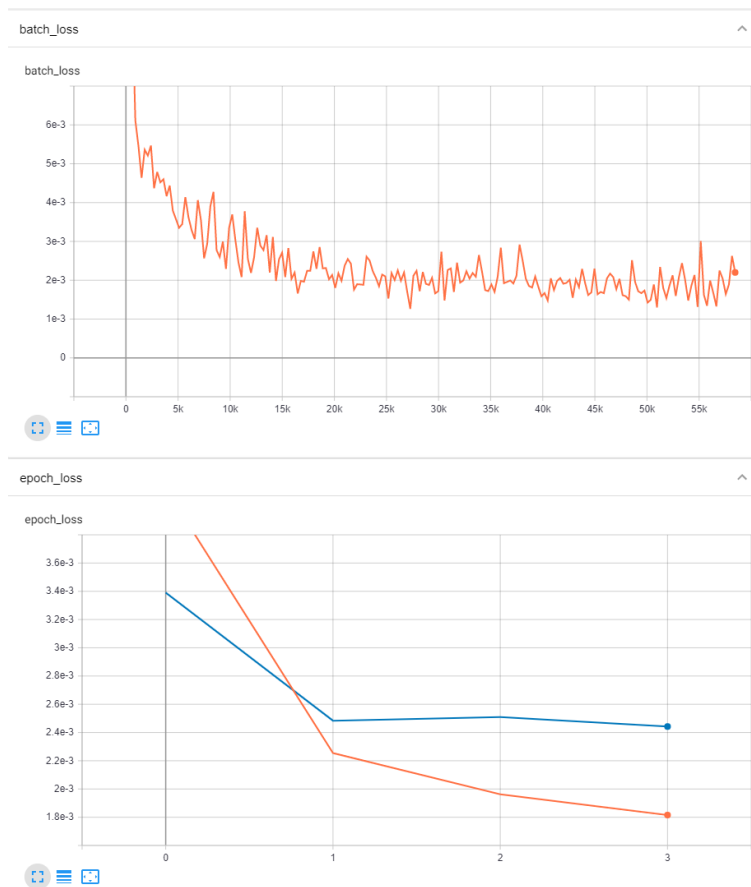
Figure 6.12: Loss value graph per batch processed (up). Loss value graph per epoch (down), where orange corresponds to training values and blue corresponds to validation values.
