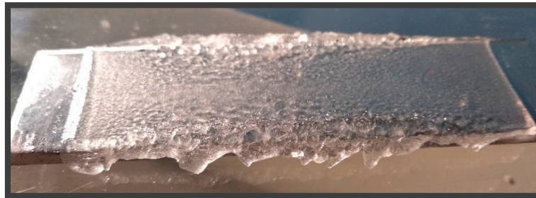
Figure 2. Glaze ice deposited on an AA6061-T6 substrate in INTA's IWT.
