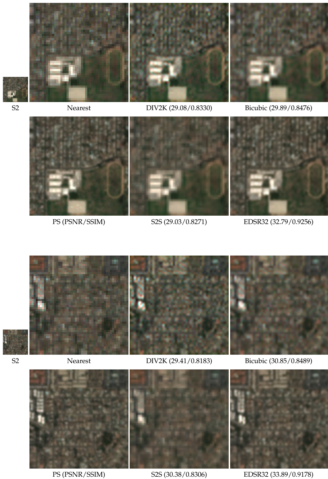
Figure 14. Visual comparison (RGB) of the baseline and EDSR32 model (tiles from test set).
