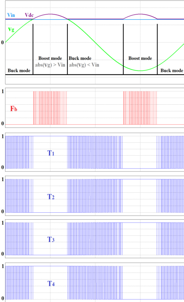
Fig. 2. Dual-mode operation principle and PWM signals.
