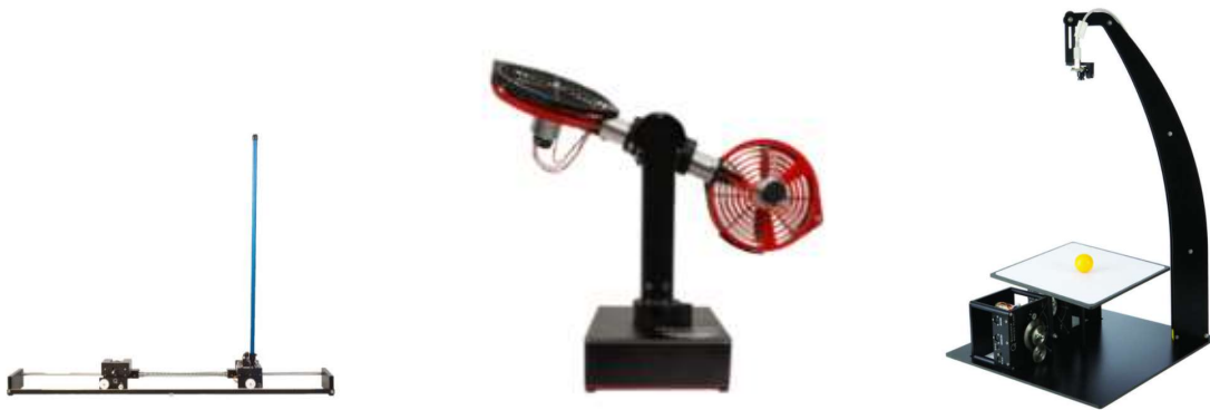
Image 4: Quanser's Inverted Pendulum [10]. Image 5: Quanser's Twin Rotor MIMO [11]. Image 6: Quanser's Ball & Plate [12].
