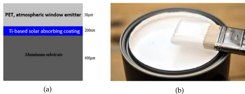
FIGURE 1.5: Radiative cooling coatings: (a) polymer radiator [9] and (b) radiative cooling paint ( TiO_2 ) [10]
