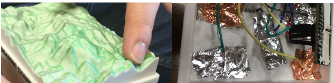
Figure 2: Left, 3D printed mountain user pointing to a peak; right, mountain is hollowed to contain electronics and sensors
