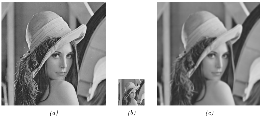
Fig. 1.3 The original image (a) is compressed with a 16 : 1 compression ratio (b). The result of applying the inverse F-Transform is shown in (c).
