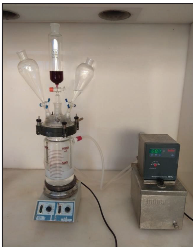
Figure I.18. Laboratory procedure for the preparation of hydrotalcites by the coprecipitation method.
