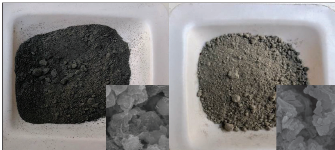
Figure I.4. Saline slags before (left) and after extraction (right).
