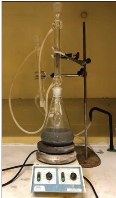
Figure I.3 Alkaline extraction of aluminum from saline slags.
