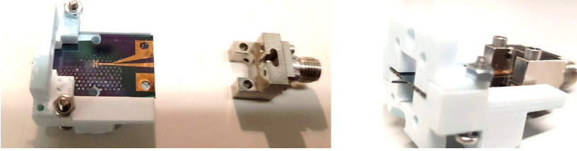
Figure 5.32: Picture of the mixer before the IF end-launcher connector assembly (left) and final assembled device (right).
