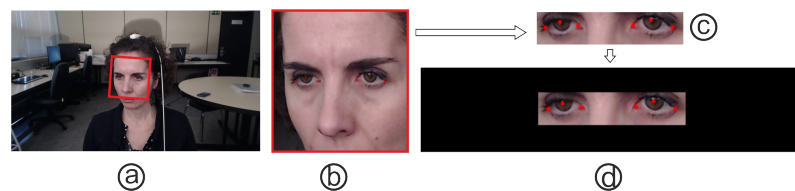
Figure 3. Image preprocessing used in the real environment experiments. The images (a) are rotated (b) so that the eyes are in the same line and cropped to the bounding box (c), which contains as meaningful information as possible. Then, a padding process (d) assures that all images have the same size before feeding them to the network. Images from the I2Head database [32].
