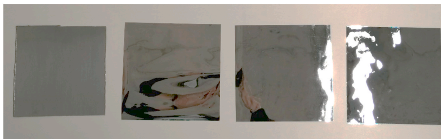
Fig. 8. Photo of the samples indicated in Table 1, from left to right: aluminum with an emissive coating (AS1), Vikuiti Substrate (V), and two samples with the emissive layer on Vikuiti ESR (VS1 and VS2).
