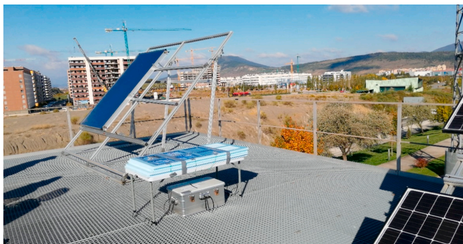
Fig. 6. Photos of the experimental setup in CENER, Sarriguren, Spain. The samples are contained in an XPS board and monitored with thermocouples connected to dataloggers.
