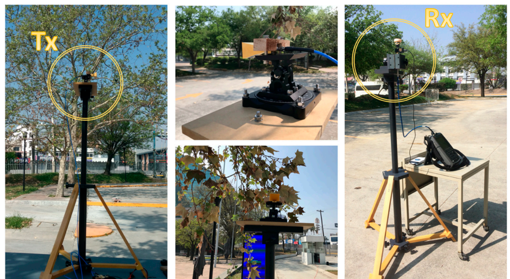
Figure 4. Transmitter and receiver experimental setup in the actual outdoor parking during the measurement campaign.
