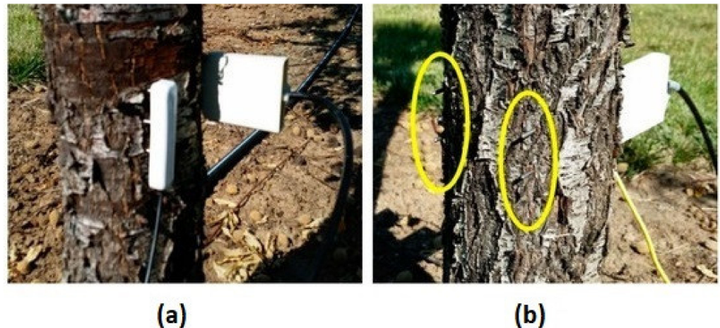
Figure 6. VSWC sensors inserted into peach tree trunks: (a) The Decagon Devices GS3 and Campbell Scientific CS655 sensors; (b) The Campbell Scientific CS655 and Acclima TDR-315L sensors [76].
