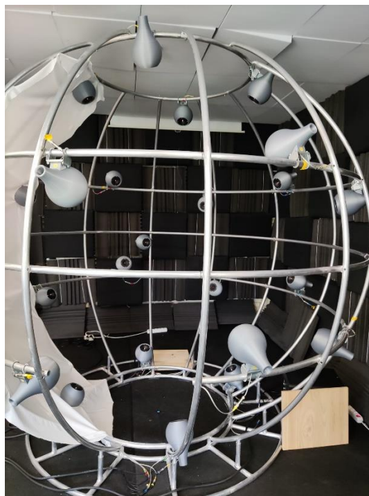
Image 1: Image of the JAULAB sphere already assembled with the 24 speakers.
