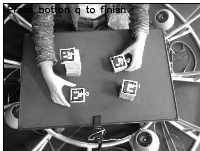
Image 15: Tokens detection during a test with real users.
