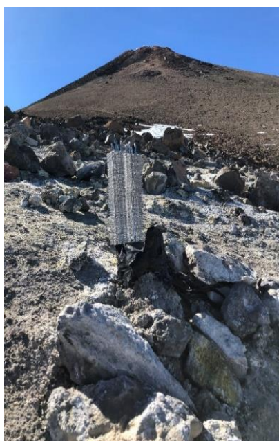
Figure 1. First thermoelectric generator installed at Teide volcano on March 2019 and its schema of operation.
