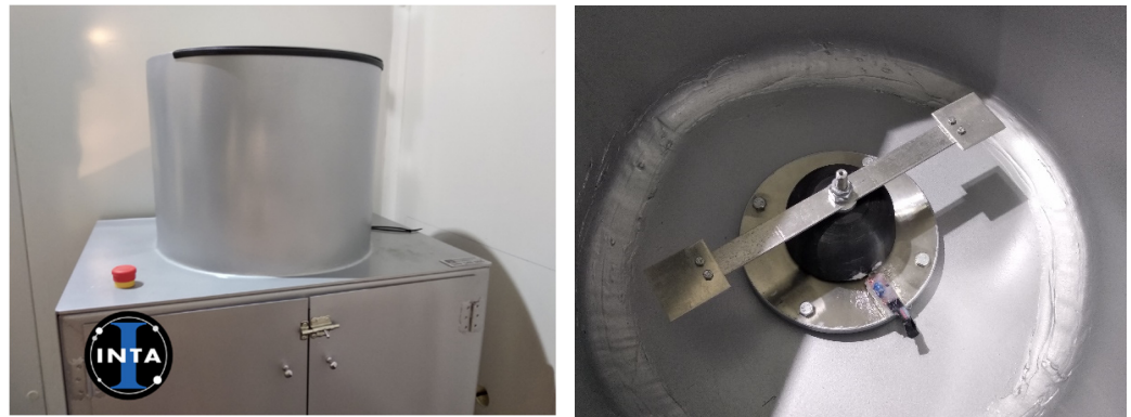
Figure 4. Centrifuge adhesion test (CAT) on a rotatory beam.
