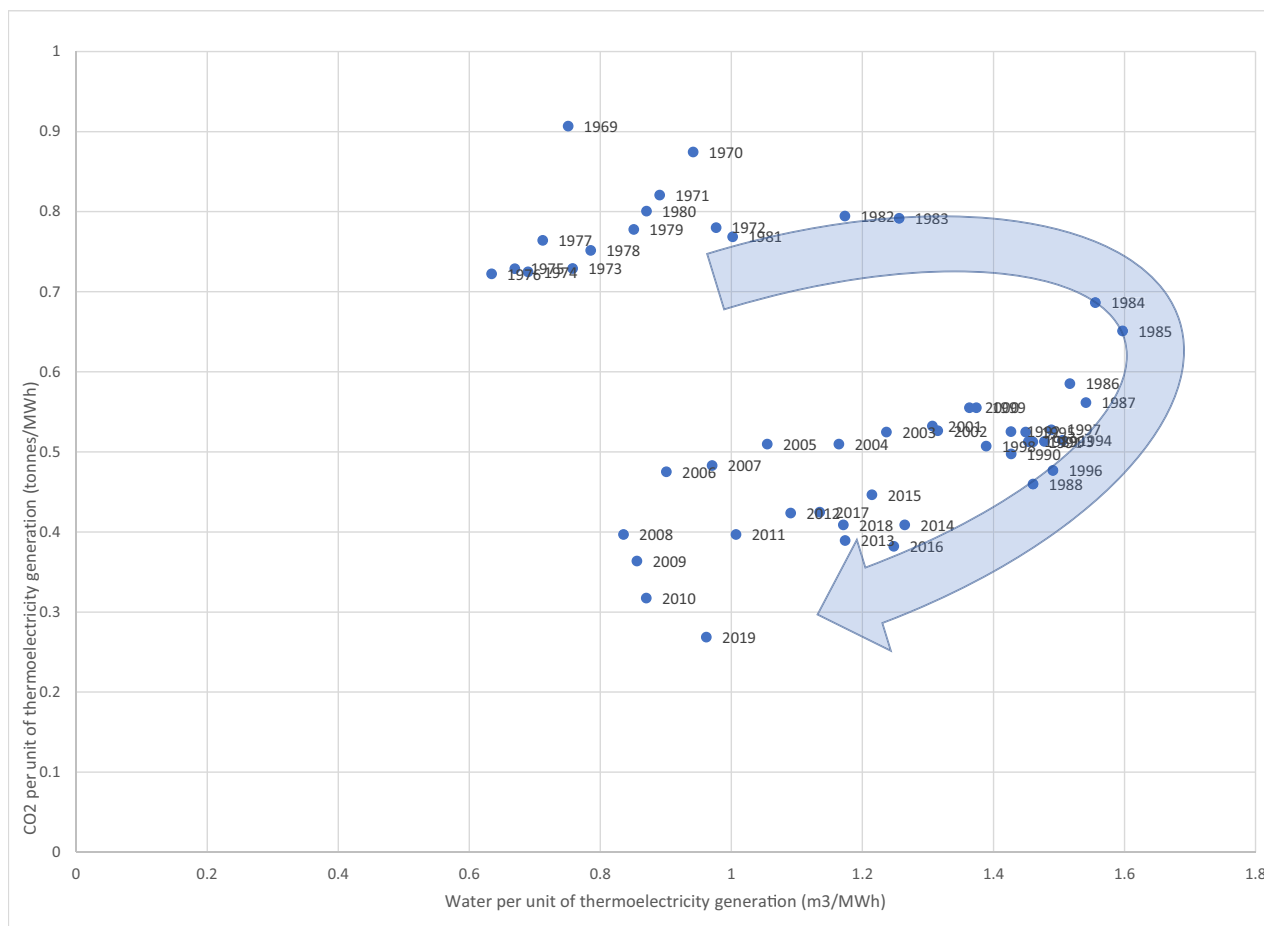
Fig. 8. Relative trade-offs: Water Consumption from thermal power (m 3 /MWh) vs Direct Carbon Emissions of thermoelectric power plants (tCO 2 /MWh) in Spain 1969–2019. Source: Figs. 5 and 6.
