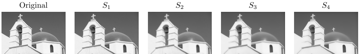
Figure 4: Original 118035 image from BSDS along with its result after image conditioning. The conditioning configurations are: Gaussian Smoothing with \sigma = 1 ( S_1 ) and \sigma = 2 ( S_2 ), and Gravitational Smoothing with the following configurations, G = 0.005, \omega_c = 20, t = 30 ( S_3 ) and G = 0.005, \omega_c = 70, t = 50 ( S_4 ).
