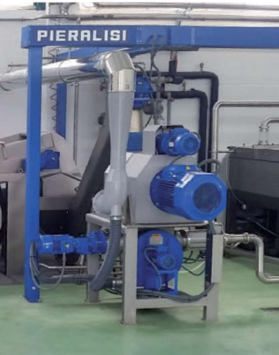
The crushing and malaxing processes are the starting point of the most delicate phases in the olive oil production process.
