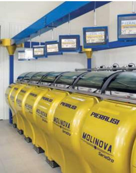
The next step in the process is called malaxation. This phase completes the development process of flavours and the organoleptic properties of olive oil started in the crushing phase. Malaxing involves slowly stirring the paste while it is thermal conditioning which causes the microscopic oil and water drops to coalesce, forming increasingly larger drops. The shape, volume and size of the paddles and the number of revolutions are key factors in obtaining the maximum yield and quality.
