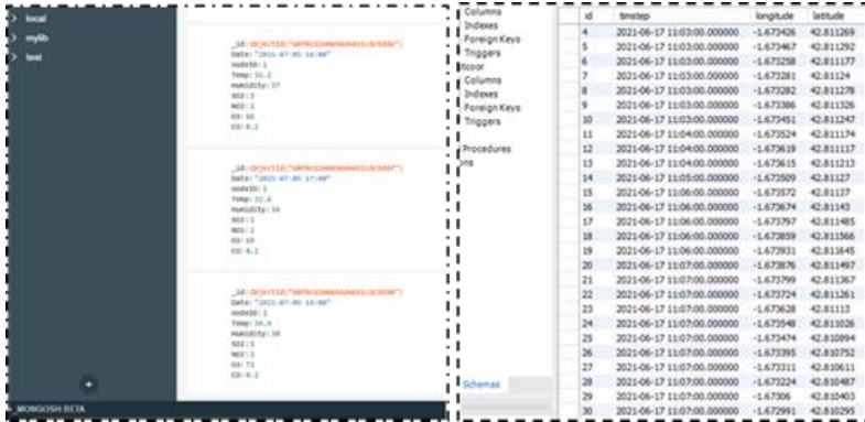
Figure 4.26: Snapshot of sensory data stored in different databases: a) MongoDB, b) MySQL.
