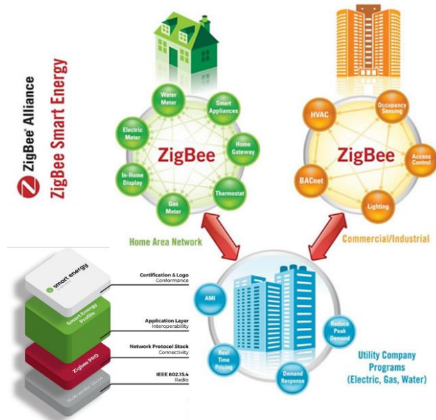
Figure 2.8: ZigBee Smart Energy wireless communication and automation (Source: Author, [94], and [95]).
