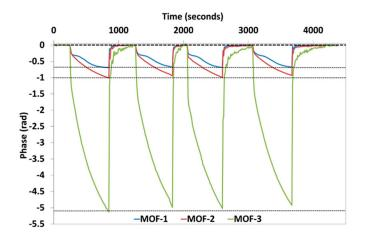
Figure 4. Phase responses of the three sensors for saturated atmospheres of ethanol.
