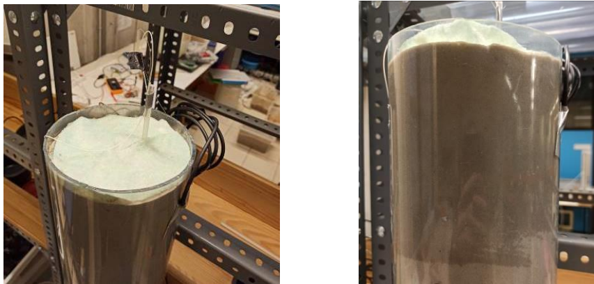
Fig. 5. Pictures of the guiding bar with the sensors sticking out from the sand-filled tube and the initial water spill.
