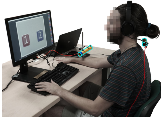
Fig. 13. Experimental setup for the user study of perception thresholds. There is an electrode above the forearm and above the nape (separation 3.5 cm). The user is in front of a computer to report the perception of the stimulus.
