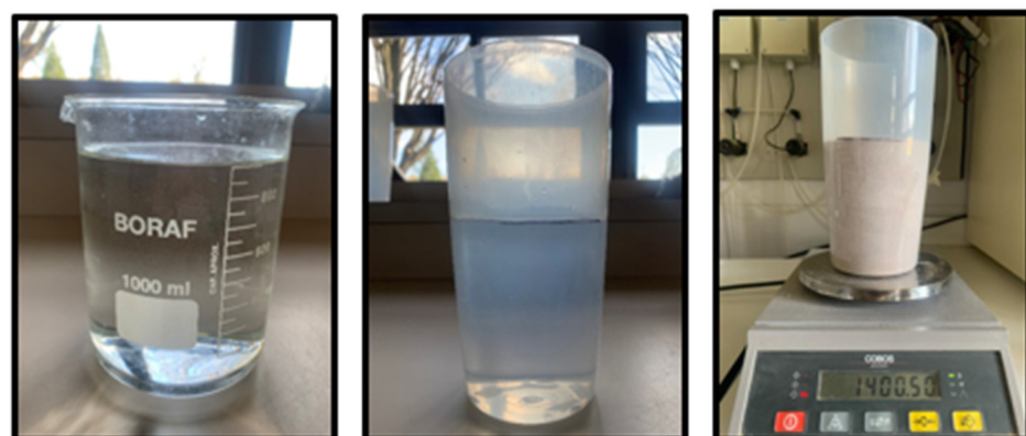
Figure 5. Steps for determining the volumetric moisture. One liter of water was measured and poured into the container where the probe measurements were placed. That volume was marked with a sharpie and filled with sand.
