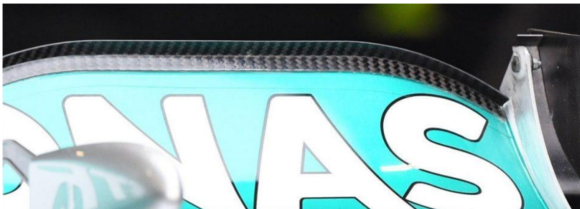
Figure 24: Gurney flap perpendicular to the upper element surface.
