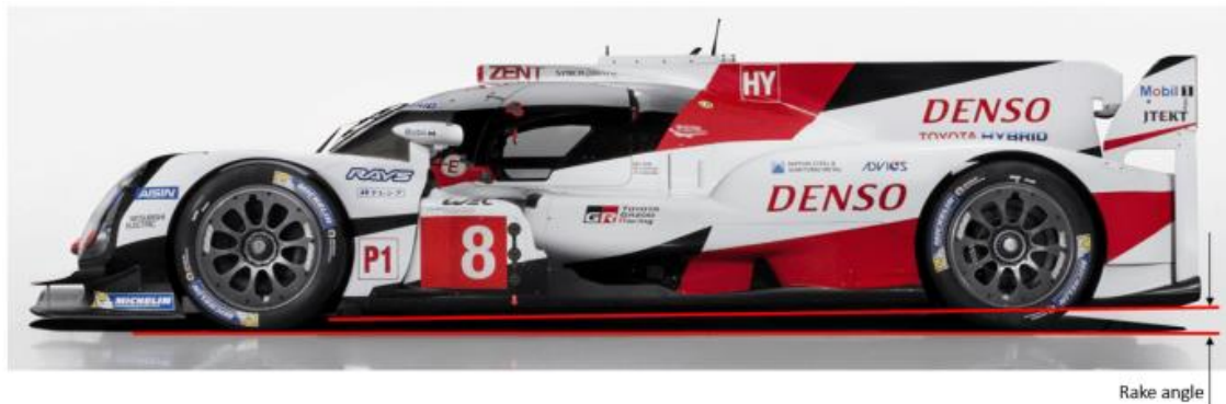
Figure 20: Rake angle in a Toyota endurance race car.
