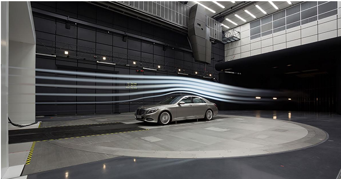
Figure 29: Automotive wind tunnel for 1:1 sized car.
