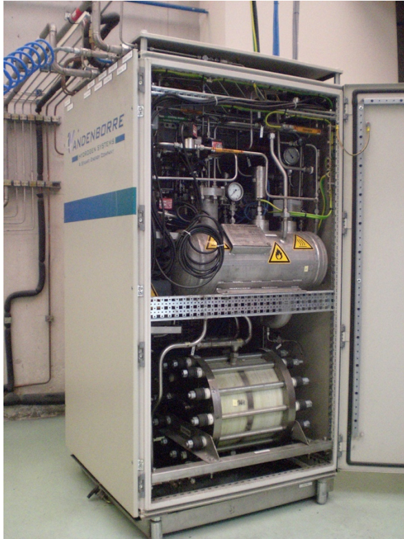
Fig. 7. Hydrogenics commercial alkaline water electrolyser H2 IGen 300/1/25.
