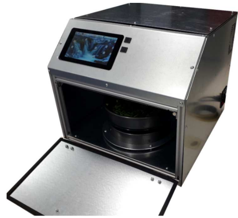
Fig. 4. Front view of the prototype developed for spectral data acquisition from alfalfa samples.
