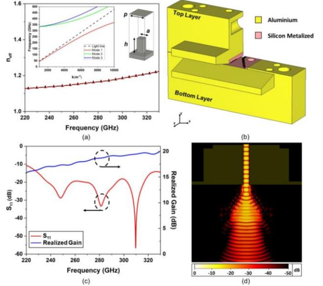
**Fig. 1.** (a) Equivalent refractive index of the pin. The inset shows a dispersion diagram of a metallic pin with the following dimensions:  $p = 0.16$  mm,  $a = 0.06$  mm and  $h = 0.121$  mm. (b) Schematic of a Hyperbolic lens system. (c) Simulated results of the structure. Magnitude of the reflection coefficient in dB and peak realized gain vs frequency. (d) Normalized electric field magnitude  $|\text{Re}\{E_z\}|$  at 310 GHz in decibel scale.
