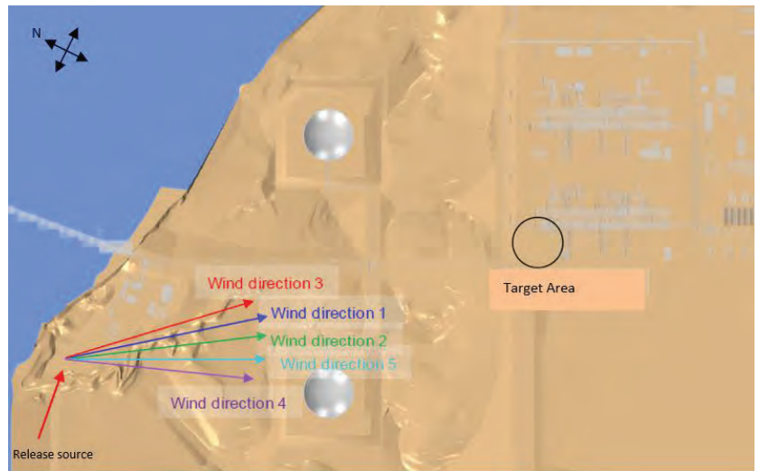
Figure 5. Schematic diagram showing the four wind directions. A target area on the first LNG train is also shown; the gas concentration calculated for this area will be used for comparison.
