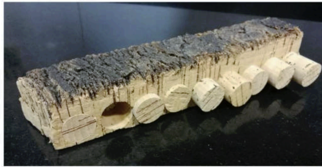
Figure 3. Punched cork stoppers (Source: authors).
