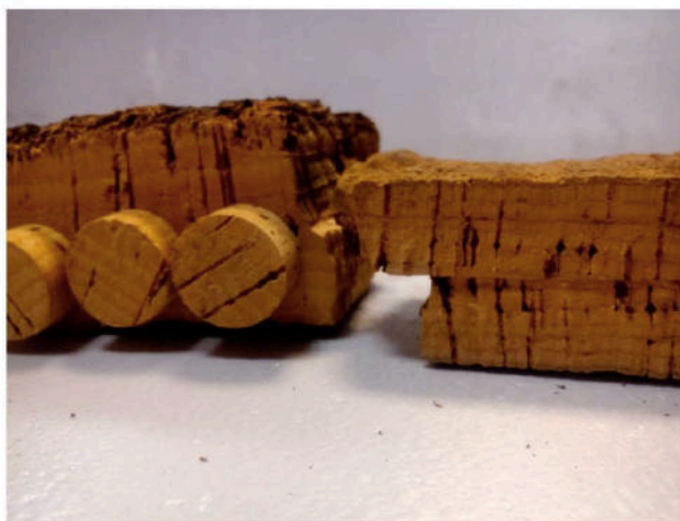
Figure 1. Perforated cork sheet to obtain one-piece stoppers on the left and 2 thin cork sheets glued together to achieve the same useful thickness and manufacture two-piece stoppers on the right.
