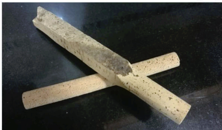
Figure 2. Turning of cork strips (Source: authors).
