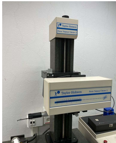
Figure 3. Taylor Hobson Talysurf 2 contact roughness meter.
