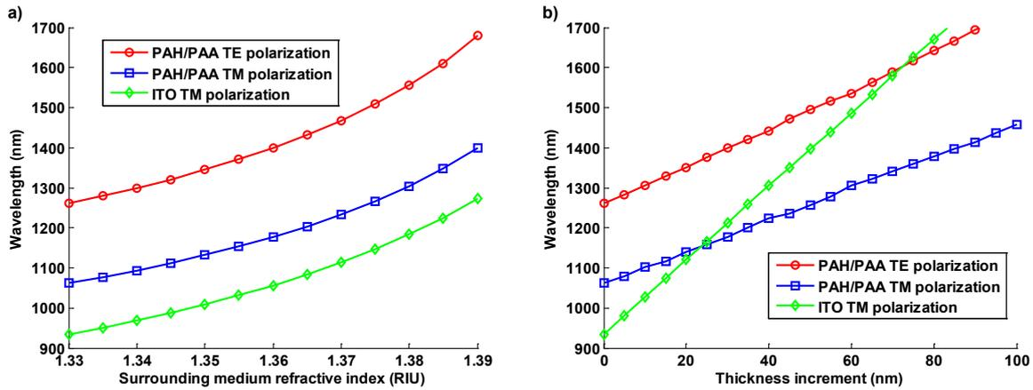
Figure 4. For PAH/PAA and ITO asymmetrically coated tapered optical fibers: a) Wavelength versus surrounding medium refractive index, b) Wavelength versus coating thickness increment
