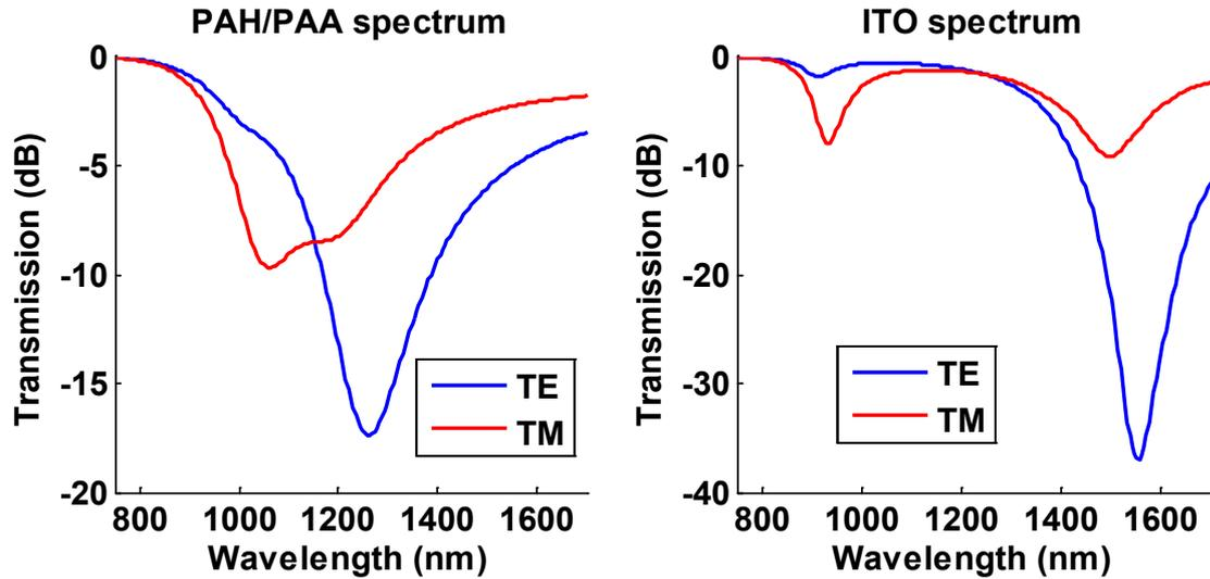
Figure 3. Spectrum for PAH/PAA and ITO asymmetrically coated tapered optical fibers. TE and TM polarization plots are included.
