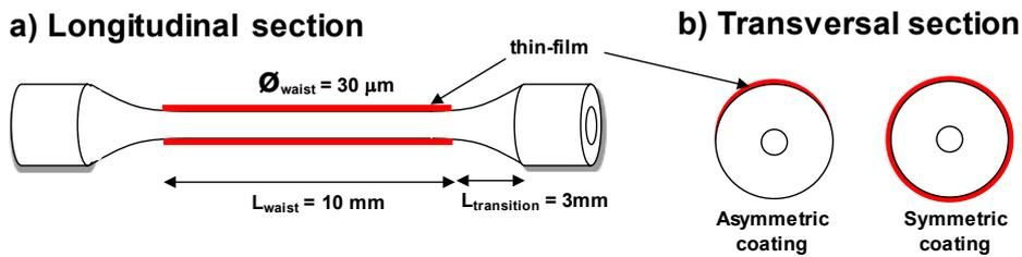
Figure 1. Longitudinal and transversal section of symmetrically and asymmetrically coated tapered optical fiber
