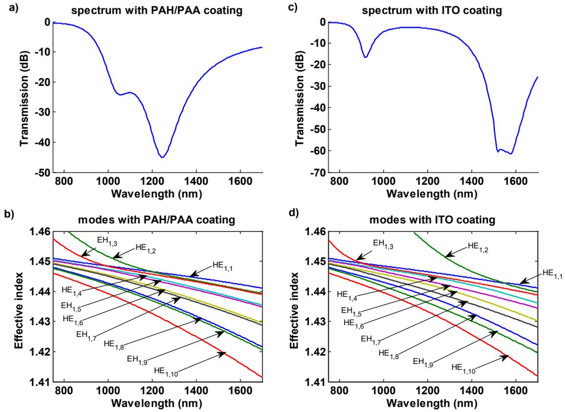
Figure 2. Spectrum and effective indices for PAH/PAA and ITO symmetrically coated tapered optical fibers
