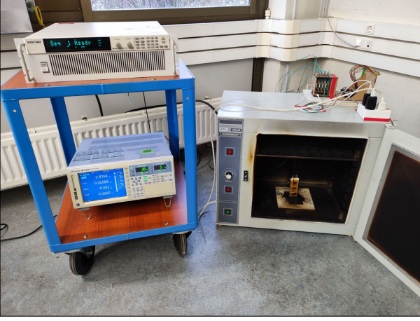
Fig. 1. Configuration of the test bench: power source and current and voltage data logger on the left, and a cell inside a resistant stainless-steel oven with temperature data logger on the right.
