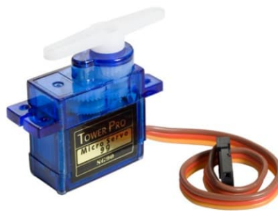
Figure 5.9: Micro Servo SG90
