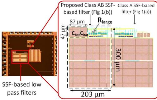
Fig. 2. Fabricated chip. An opaque passivation layer was applied on top of IC. Thus, only capacitors are discernible in the chip photo (on the left). At the right, there is a zoom area with the layout.
