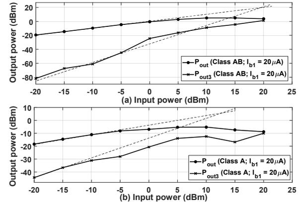
Fig. 6. Measured IP3 at 350 kHz with  $I_{b1} = 20 \mu\text{A}$  for (a) the class AB SSF filter (IIP3 = 18 dBm; OIP3 = 20 dBm) and (b) the class A SSF filter (IIP3 = 13 dBm; OIP3 = 5.5 dBm)
