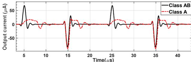
Fig. 8. Measured output current of the proposed class AB filter and its class A counterpart to a 50 kHz square input signal.
