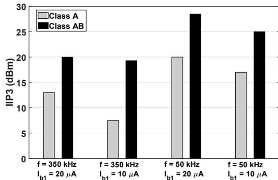
Fig. 7. Comparison of IP3 values in different frequency ranges and bias conditions between the class A SSF filter and the proposed class AB SSF filter.
