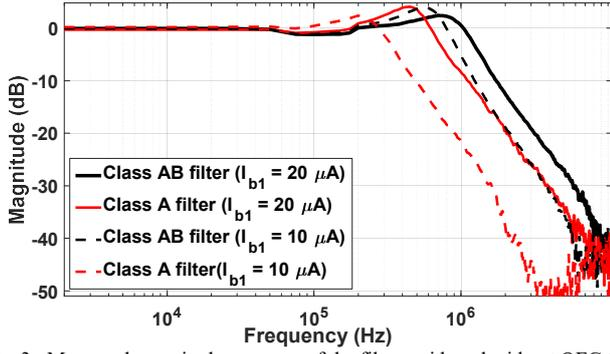
Fig. 3. Measured magnitude response of the filters with and without QFG for a reference bias current  $I_{b1}$  of 20  $\mu\text{A}$  and (b) 10  $\mu\text{A}$ .
