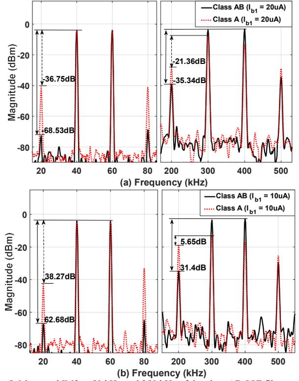
Fig. 5. Measured IM3 at 50 kHz and 350 kHz of the class AB SSF filter (straight line) and class A SSF filter (dotted line) for a reference bias current  $I_{b1}$  of (a) 20  $\mu\text{A}$  and (b) 10  $\mu\text{A}$ .
