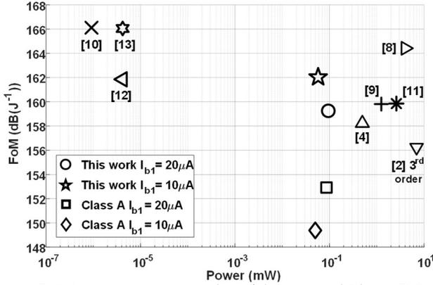
Fig. 9. FoM1 vs. power consumption of the proposed Class AB SSF filter (for bias currents of 10  $\mu$ A and 20  $\mu$ A) compared to the fabricated Class A version of the filter and previous works.
