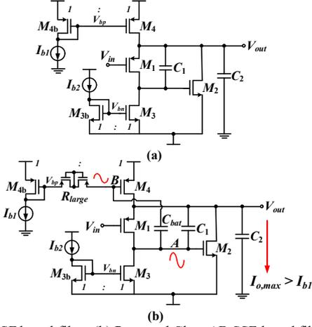
Fig. 1. (a) SSF based-filter (b) Proposed Class AB SSF-based filter.
