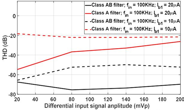
Fig. 4. Measured THD values of the class A and class AB SSF filters for an input signal of 100 kHz and different amplitude values for a reference bias current  $I_{b1}$  of (a) 20  $\mu\text{A}$  and (b) 10  $\mu\text{A}$ .
