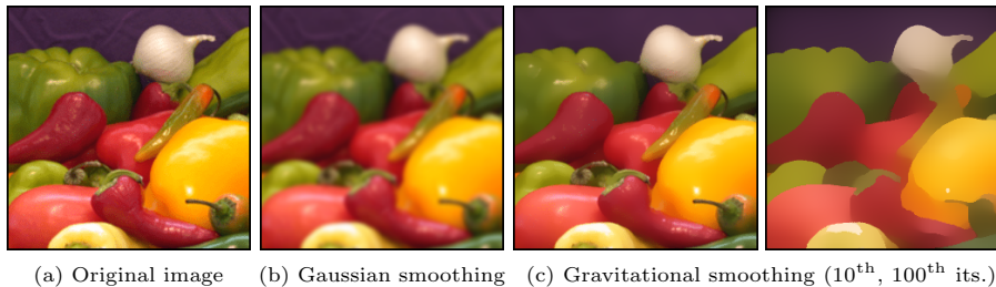
Fig. 1. Example of image smoothing performed with content-aware and content-unaware techniques. (a) The original image; (b) the result with content-unaware smoothing (Gaussian smoothing, \sigma = 2 ); (c) the smoothing output from the 10 th and 100 th iteration of gravitational (content-aware) smoothing, respectively. For CUS, (b) shows the blurring of the edges and loss of information. For CAS, (c) shows the progressive blending of tones within objects, while preserving their boundaries.
