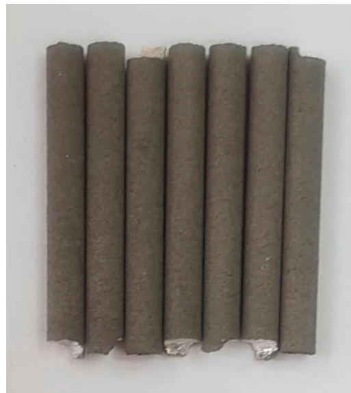
Figure 5. Temporary demonstrative implants realised via SLM from Mg-10Zn-0.8Ca-0.5Zr biodegradable alloy.
