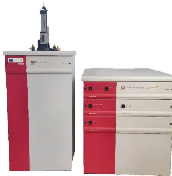
Fig. 2.7. Quantum Design MPMS XL-7 SQUID magnetometer.
