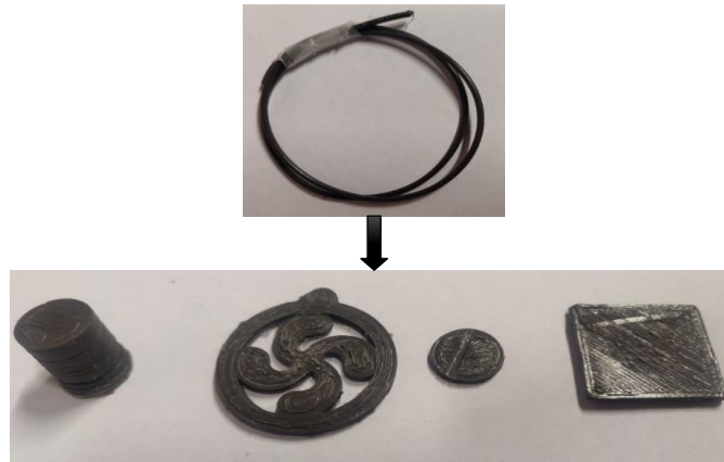
Fig. 5.19. Polymer-composite wire and 3D-printed objects with P_{0-100}^{50}MP^{50} .
