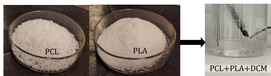
Fig. 5.4 . Raw polymers PCL, PLA, and c) mixing of PLA, PCL and DCM with magnetic stirrer.
