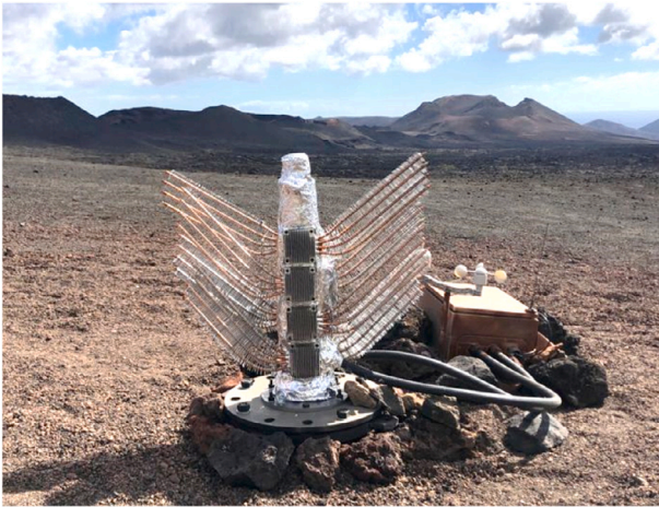
Fig. 3. Geothermal thermoelectric generator for high temperature geothermal anomalies installed in Islote Hilario , Timanfaya National Park [23].
