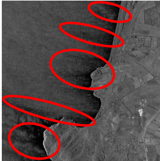
Figure 5.2.5.11 Equalized image of the image 2. It has been equalized in order to make visible the features to detect. The red circles denote that there are bright points in the original image, that is waves or current changes.
