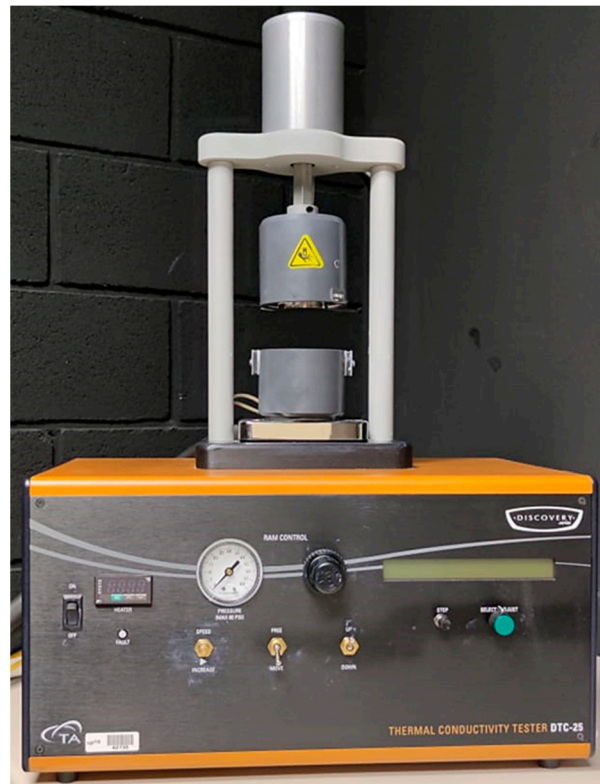
Figure 1. Test bench DTC-25 [24].
