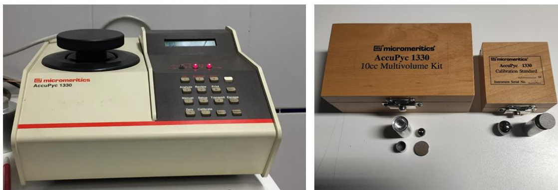
Figure 2.13. (left) AccuPyc 1330 Helium pycnometer, and (right) multivolume kit and calibration standards for skeletal density measurements. The instrument and components are located in the Science Department of the Public University of Navarre.
