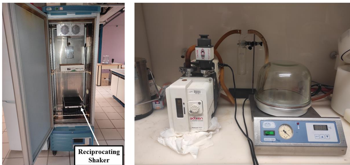
Figure 2.3. J.P. Selecta S.A thermostatised oven ( left ), and Selecta S.A heating plate connected to an adixen Pfeiffer vacuum pump ( right ). The apparatuses are located in the Science Department of the Public University of Navarre.
