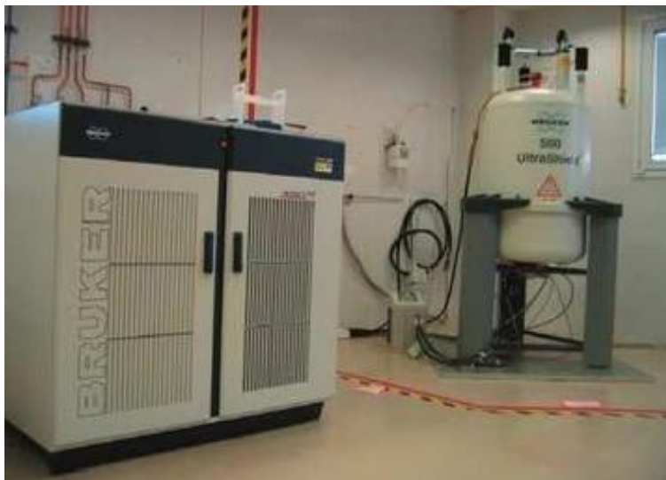
Figure 2.7. Bruker AV-400 MHz solid-state nuclear magnetic resonance spectrometer (SCAI of the University of Jaén).
