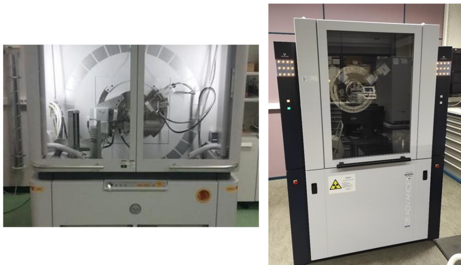
Figure 2.12. X-ray diffractometers: ( left ) PANalytical Empyrean XRD in the SCAI of the University of Jaén, and ( right ) Bruker D8-Advance powder XRD instrument in the UCTAI of the Public University of Navarre.
