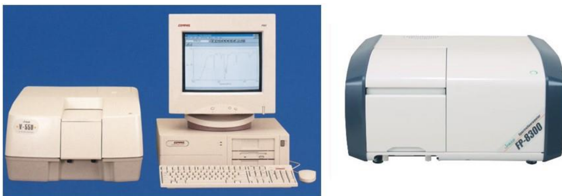
Figure 2.10. Spectrometers used at the Faculty of Engineering of the University of Porto: ( left ) Jasco UV-Vis spectrometer mod V-560, image subtracted from the manual of the equipment available online; and ( right ) Jasco spectrofluorometer mod FP-8300, image downloaded from the Jasco.co.uk webpage.
