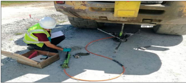
Figure 7. Field bearing plate testing procedure.
