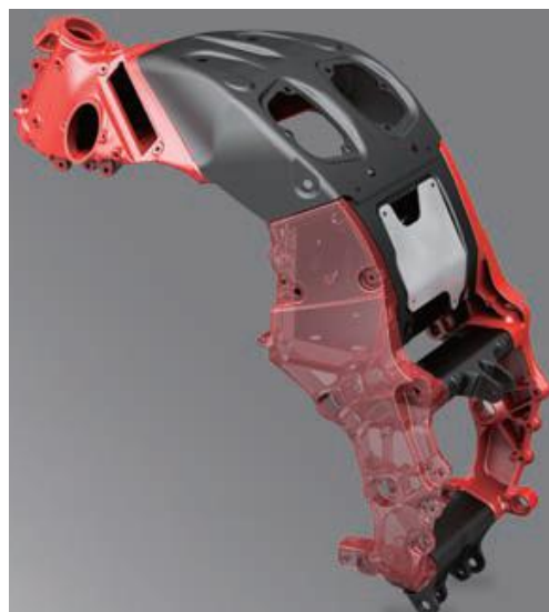
Figura 47. Chasis Monocasco, Kawasaki ZZR 1400 (2012)
