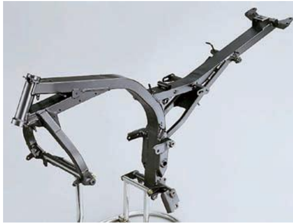
Figura 48. Chasis monoviga, Honda CB 900F (2002)
