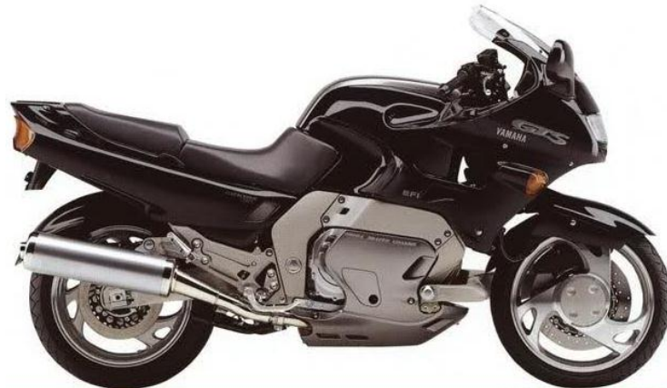
Figura 49. Chasis Omega, Yamaha GTS 1000 (1993)
